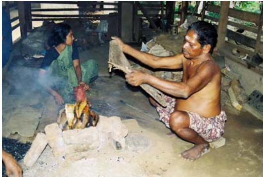
Mirrors: Metal Mirrors from India. Fig. 3 Heating of crucible-cum-mould in a hearth fuelled by coconut husks.
